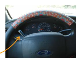
There are two control switches; a push button on the end of the stick and a slide switch you can see in the photo. This cruise control works just like most others: turn on the cruise control, set to the speed you want, speed up/ slow down, and turn off the system.
