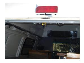
A backup camera has been installed above the rear doors, below the third brake light, that is pointed slightly downward.
